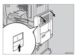
While lifting the lever, lift cover Z1 (1), and remove the misfed paper (2).
