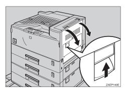
2 Open the upper right cover by pulling the handle, and remove the misfed paper.
