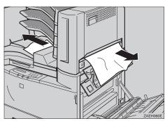
If the misfed paper is not removed in step **E**, open the upper cover of the bridge unit, and remove the misfed paper.
