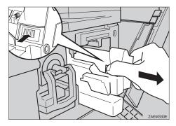
Raise the green handle and slide the photo conductor unit out towards you.
